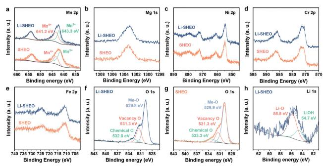
Fig. 3 High-resolution XPS spectra of Li-SHEO and SHEO: (a) Mn 2p, (b) Mg 1s, (c) Ni 2p, (d) Cr 2p, (e) Fe 2p, (f), (g) O 1s, and (h) Li 1s.
