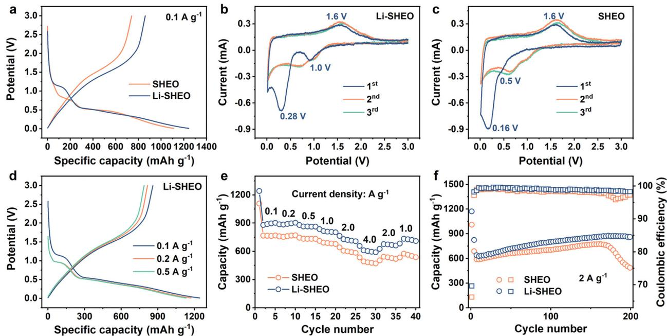
Fig. 4 Electrochemical performance of the  $\text{Li}_2\text{O}$ -doped SHEO anode: (a) initial discharge–charge profile of the Li-SHEO and SHEO anodes under  $0.1 \text{ A g}^{-1}$ , CV curves of (b) Li-SHEO and (c) SHEO anodes, (d) initial discharge–charge curves of the Li-SHEO anode under  $0.1$ ,  $0.2$ , and  $0.5 \text{ A g}^{-1}$ , (e) rate capability and (f) cyclic property with related Coulombic efficiency of the Li-SHEO and SHEO anodes.
