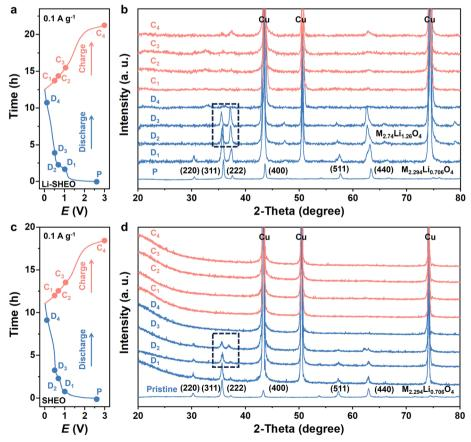
Fig. 5 The ex situ XRD of the Li-SHEO and SHEO anodes recorded during the initial cycle: (a) and (c) the related discharge-charge profile and (b) and (d) ex situ XRD patterns.  $D_1-D_4$  represent discharged to 1.0 V, 0.8 V, 0.5 V, 0.1 V, respectively;  $C_1-C_4$  represent charged to 0.5 V, 0.8 V, 1.0 V, 3.0 V, respectively.
