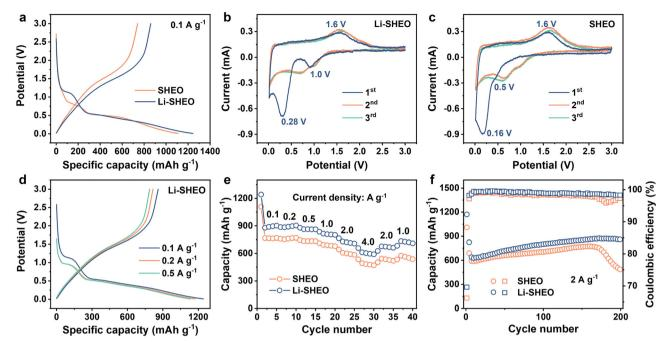
Fig. 4 Electrochemical performance of the Li<sub>2</sub>O-doped SHEO anode: (a) initial discharge-charge profile of the Li-SHEO and SHEO anodes under 0.1 A g<sup>-1</sup>, CV curves of (b) Li-SHEO and (c) SHEO anodes, (d) initial discharge-charge curves of the Li-SHEO anode under 0.1, 0.2, and 0.5 A g<sup>-1</sup>, (e) rate capability and (f) cyclic property with related Coulombic efficiency of the Li-SHEO and SHEO anodes.
