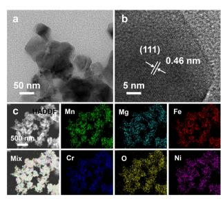
Fig. 2 (a) TEM and (b) HR-TEM image, as well as (c) HADDF image with the related EDS mapping results of Li-SHEO material.
