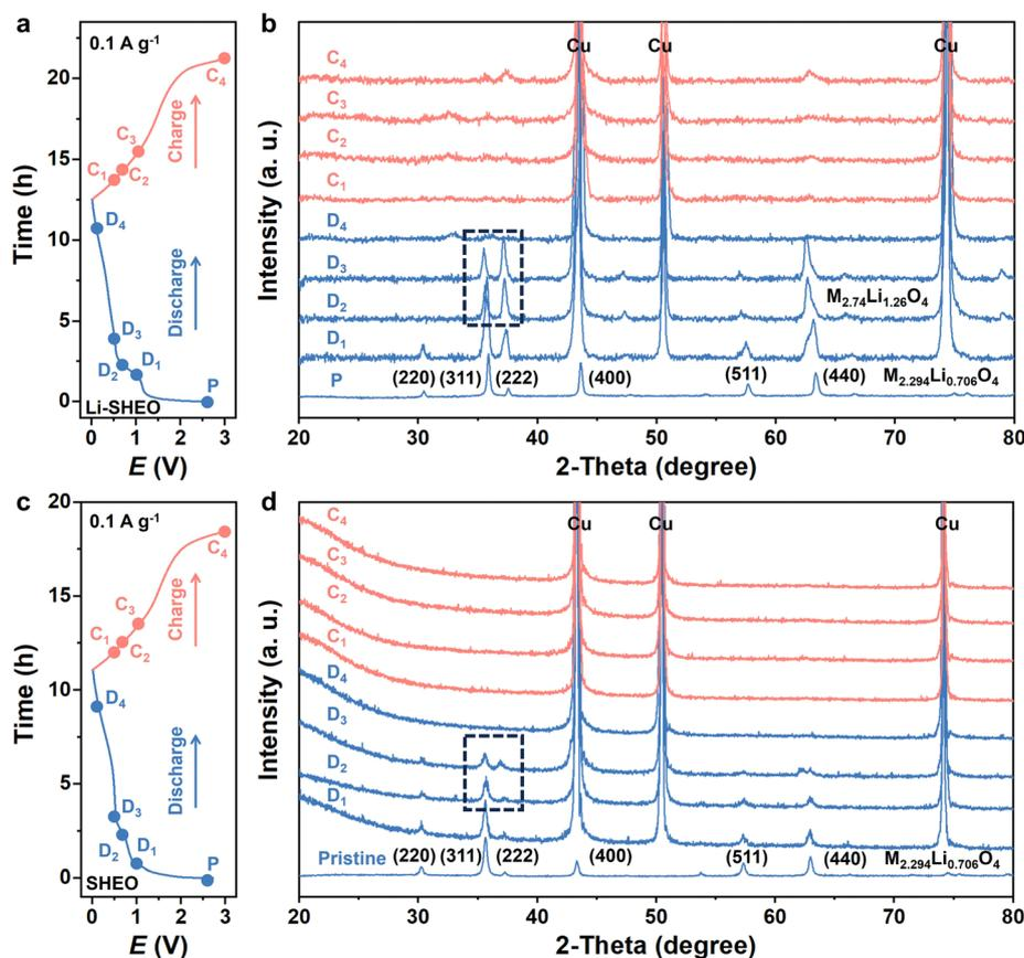
Fig. 5 The *ex situ* XRD of the Li-SHEO and SHEO anodes recorded during the initial cycle: (a) and (c) the related discharge–charge profile and (b) and (d) *ex situ* XRD patterns. D<sub>1</sub>–D<sub>4</sub> represent discharged to 1.0 V, 0.8 V, 0.5 V, 0.1 V, respectively; C<sub>1</sub>–C<sub>4</sub> represent charged to 0.5 V, 0.8 V, 1.0 V, 3.0 V, respectively.
