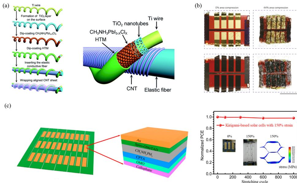
Fig. 3 (a) Schematic illustration of the elastic PSC fibre;<sup>53</sup> (b) schematic of the ultrathin and buckling FPSCs;<sup>54</sup> (c) schematic illustration of the kirigami-based PSC array and structure of PSCs and normalized PCE of kirigami-based PSCs after different stretching cycles.<sup>55</sup>
