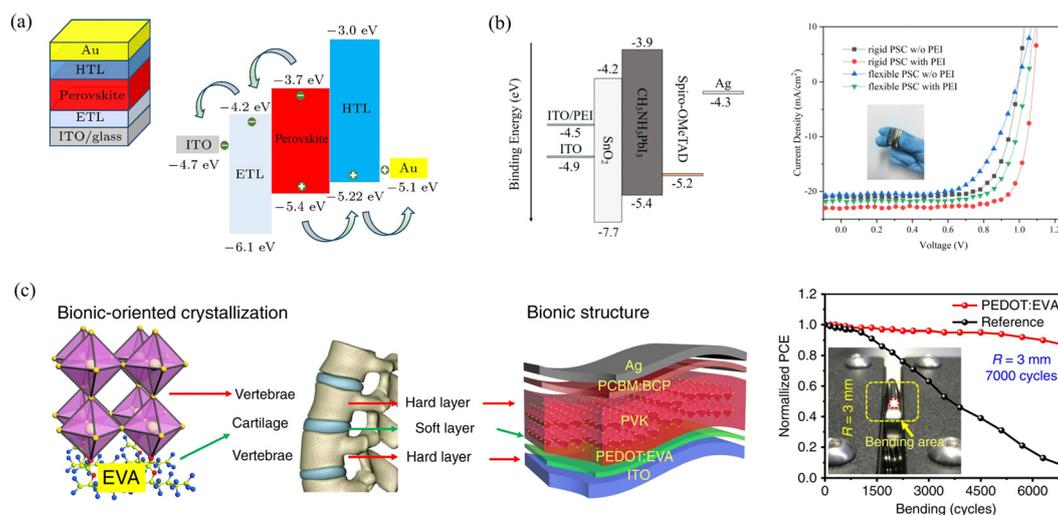
Fig. 2 (a) Structure and energy band diagram of perovskite solar cell;<sup>44</sup> (b) the energy levels of the materials used in the devices and the  $J$ - $V$  curves of the champion devices with and without PEI;<sup>43</sup> (c) biomimetic mechanisms of the vertebrae and PSCs and normalized averaged PCE value for the flexible PSCs under bending cycles with radius of 3 mm.<sup>46</sup>
