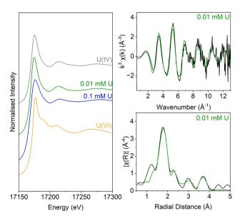
Fig. 5 U  $L_{III}$ -edge spectra for solids from the low (0.005 mM) U and middle (0.05 mM) U samples. These samples are compared with U(vi) (aqueous U(vi)-triscarbonate) and U(vi) (uraninite) standards taken from previous work (Roberts *et al.*, 2017; Townsend *et al.*, 2020). Right: U  $L_{III}$ -edge XAS spectra for NB1. Top - k3-weighted EXAFS. Bottom - Fourier transform of k3-weighted EXAFS, using a Hanning window function.
