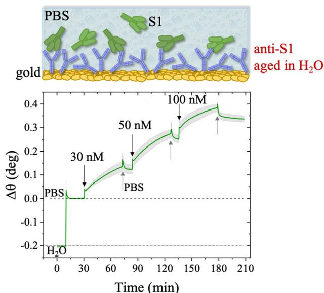
**Fig. 9** S1 Sensogram of an anti-S1 layer, kept for 24 h in water. The experiment was performed in the S1 range of concentrations 30 nM–100 nM. The green trace is the average of the SPR signals registered by sampling the anti-S1 layer in two different points, 3 millimeters apart, along with the relative standard deviation. Black and grey arrows specify the times of the injections into the SPR flow-through cell for S1 standard solutions and PBS washing step, respectively.
