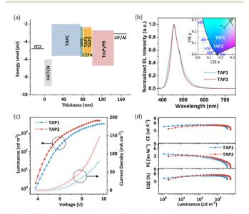
(a) Energy level diagram; (b) electroluminescent spectra (inset shows the corresponding CIE coordinates); (c) luminance-voltagecurrent density plots and (d) efficiency-luminance characteristics of the blue OLEDs.
