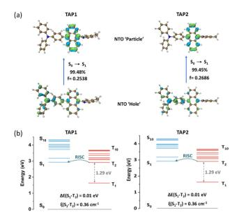
Fig. 3 (a) NTO distributions for the  $S_0 \rightarrow S_1$  transition and (b) energy level diagrams including SOC constants (ξ) of TAP1 (left) and TAP2 (right).
