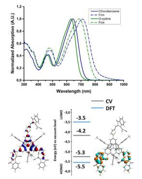
Absorption spectra of AzaTk in solution and in thin films. Energy levels and electron density of the HOMO (left) and LUMO (right) of AzaTk obtained by cyclic voltammetry and DFT calculations
