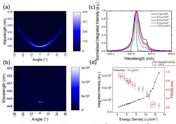
Fig. 4 Planar microcavity Fourier imaging PL dispersion (a) below threshold at 6 μJ cm<sup>-2</sup> (b) after threshold (11 μJ cm<sup>-2</sup>) (c) emission spectra narrowing captured at k = 0, as a function of energy density (d) input-output characteristics for planar cavity, where integrated intensity (left) and FWHM (right) is plotted as a function of energy density
