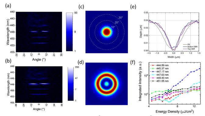
Fig. 5 Defect microcavity dispersion (a) below threshold (7.7  $\mu$ J cm<sup>-2</sup>) (b) above threshold (12.0  $\mu$ J cm<sup>-2</sup>), Numerical simulation of the far-field projection for cylindrical defect (c) lowest energy mode (d) lasing mode (e) Defect profile for each layer of the microcavity, measured with AFM (f) Integrated intensity extracted from the Fourier imaging dispersion as a function energy density for each emitting mode with lasing coming from 447.17 nm.
