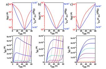
Fig. 7 Typical n-type field-effect transistor transfer (top) and output (bottom) characteristics for polymers P2 (a), P3 (b) and P4 (c). The transfer characteristics were measured at a  $V_{\rm DS}$  of 80 V. The output curves were measured at a  $V_{\rm G}$  from 0 to 80 V in intervals of 10 V and over a  $V_{\rm DS}$  range of 0 to 80 V
