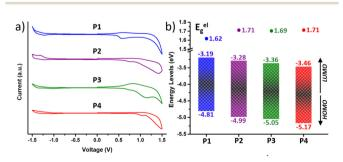
Fig. 4 (a) Cyclic voltammograms as a thin film (scan rate  $100 \text{ mV s}^{-1}$ ) and (b) HOMO-LUMO energy levels of the copolymers P1-P4
