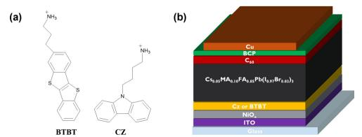
Fig. 1 (a) Molecular structure of BTBT and Cz. (b) Perovskite solar cell stack depiction. The control sample does not contain any modification between NiOx and the perovskite laver
