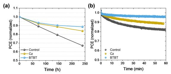
Stability test on PSCs without encapsulation in (a) ambient conditions (25% RH) and (b) under continuous illumination and MPPT conditions
