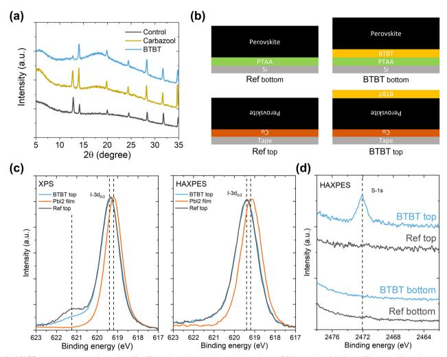
Fig. 4 (a) XRD measurements performed on lift-off samples with and without the interlayers. (b) Illustration of the four different configurations used for XPS and HAXPES measurements. (c) XPS and HAXPES measurements performed on lift-off samples concentrating on the I-3d<sub>5/2</sub> core level. (d) HAXPES measurement performed on all configurations concentrating on the S-1s core level.
