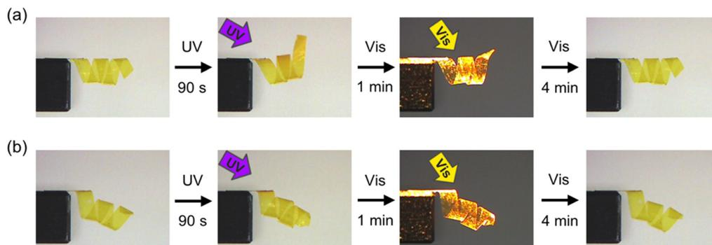
**Fig. 3** Photoinduced deformation behaviours of PAzo/PMMA IPN samples with spiral shapes upon irradiation with UV ( $365\text{ nm}$ ,  $20\text{ mW cm}^{-2}$ ) and visible light ( $>540\text{ nm}$ ,  $40\text{ mW cm}^{-2}$ ). (a) In-plane uniaxial alignment. (b) Homeotropic alignment. Original sizes of the films:  $20\text{ mm} \times 1\text{ mm} \times 8\text{ }\mu\text{m}$ .
