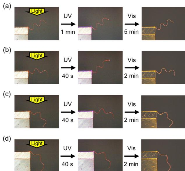
Fig. 4 Photoinduced deformation behaviours of a PAzo/PMMA IPN film with a wavy shape at (a) room temperature, (b) 100 °C, (c) 120 °C and (d) 140 °C. UV: 15 mW cm<sup>-2</sup>. Vis: 10 mW cm<sup>-2</sup>. The original size of the film: 20 mm × 1 mm × 19 μm.
