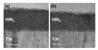
Fig. 8 Cs-STEM image of HfN $_{x}$  annealed at (a) 450 °C and (b) 700 °C. All films were deposited with pre-cleaning step.
