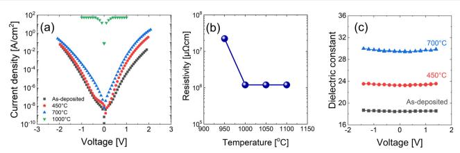
Fig. 7 (a) Current density-voltage graph, (b) resistivity, and (c) dielectric constant-voltage analysis of 15 nm  $HfN_x$  films annealed at various temperatures under  $NH_3$  ambient.
