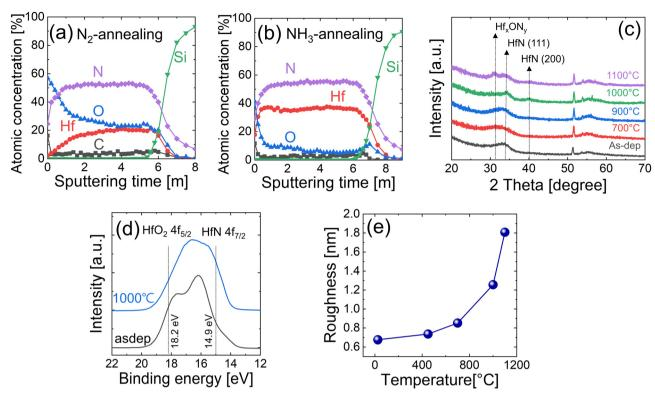
Fig. 4 AES depth profile of the  $HfN_x$  film annealed at 900 °C with (a)  $N_2$  and (b)  $NH_3$  ambient. (c) Grazing-angle incidence X-ray diffraction (GIXRD) analysis of films annealed at various temperatures, X-ray photoelectron spectroscopy of films annealed at various temperatures, and (e) roughness. All films were deposited with the precleaning step, with a thickness of 15 nm, and annealing was conducted in  $NH_3$  ambient, except for (a).
