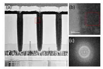
Fig. 5 (a) Cs-corrected scanning transmission electron microscopy (Cs-STEM) image of HfN<sub>x</sub> film deposited on contact hole structure with an aspect ratio of 1:7, (b) Cs-corrected TEM image of red square area in (a) and (c) fast-Fourier transformed image of red box area in (b).
