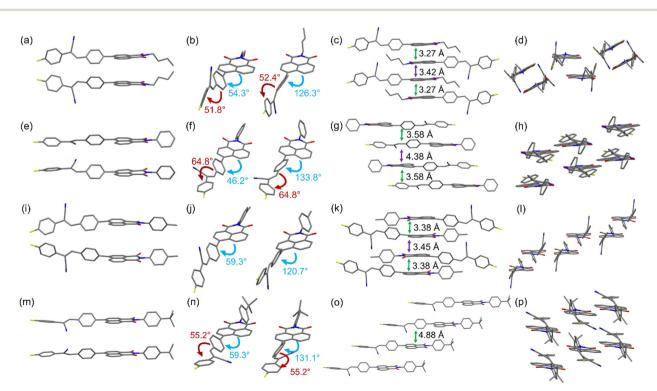
Fig. 5 Molecular conformation and packing structures derived from single-crystal structure analysis of NICSF-B (a-d), NICSF-P (e-h), NICSF-M (i-l), and NICSF-T (m-p).
