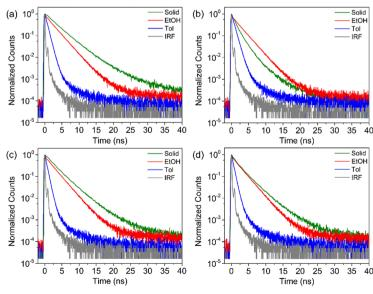
Fig. 3 Normalized TCSPC plots of (a) NICSF-B, (b) NICSF-P, (c) NICSF-M and (d) NICSF-T in Tol (blue), EtOH (red) and in the aggregated state (green), the gray curves present the instrument response functions (IRF)
