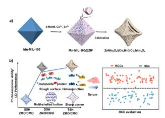
Scheme 1 Schematic illustration of the (a) synthetic route to tripleshelled ZnMn<sub>2</sub>O<sub>4</sub>/(Co, Mn)(Co, Mn)<sub>2</sub>O<sub>4</sub> (TSH ZMO/CMO) and (b) LDI-MS extraction of serum metabolic fingerprints by TSH ZMO/CMO with specific physical effects for evaluation of hepatocellular carcinoma (HCC).
