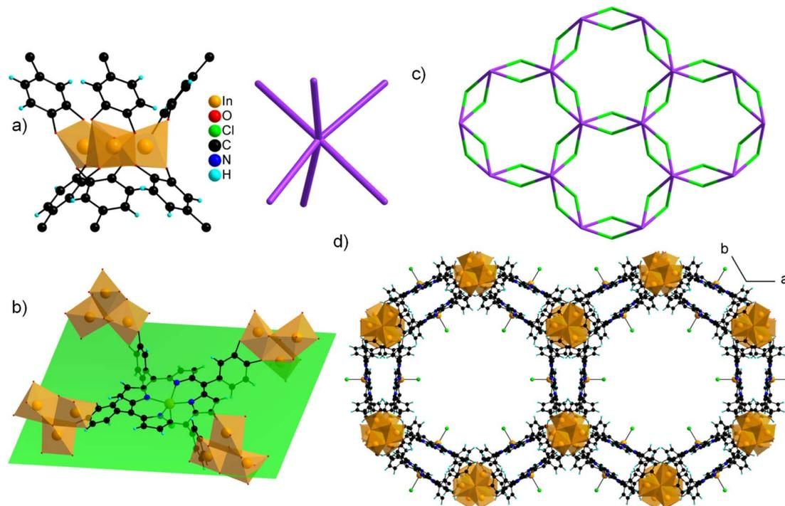
Fig. 9 Crystal structure of **3(In)**. (a) Inorganic secondary building unit (left) acting as a distorted octahedron (right); (b) InClTcatPP ligand surrounded by four inorganic SBUs, with the mean plane of the macrocycle shown in green; (c) distorted **stp** net (the ligand and the inorganic SBU are shown in green and violet, respectively); (d) full structure showing the channels running along the *c*-axis.
