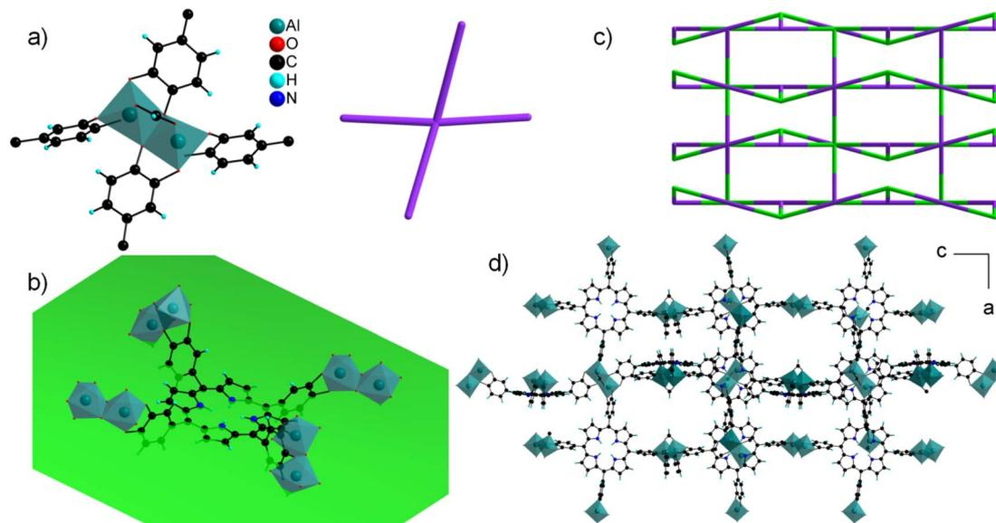
Fig. 8 Crystal structure of CatPMOF-2(Al). (a) Inorganic SBU (left) acting as a distorted square planar node (right); (b)  $\text{H}_2\text{TcatPP}$  ligand, with the mean plane of the macrocycle shown in green; (c) cds net (the ligand and the inorganic SBU are shown in green and violet, respectively); (d) full structure shown along the  $b$  axis.
