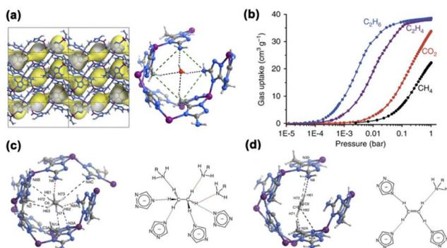
Fig. 6 (a) Crystal structure of MAF-49, showing a water molecule in the molecular pocket. (b) Single-component adsorption isotherms of  $C_2H_6$ ,  $C_2H_4$ ,  $C_2H_2$ , and  $CO_2$  on MAF-49 at 316 K. Crystal structure of (c)  $C_2H_6@MAF-49$  and (d)  $C_2H_4@MAF-49$ , highlighting the multiple binding interactions. Reproduced from ref. 51 with permission from copyright 2015, Springer Nature.
