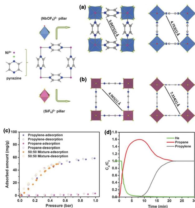
Fig. 11 Comparison of the building block arrangement of (a) KAUST-7 and (b) SIFSIX-3-Ni. (c) Adsorption isotherms of  $\text{C}_3\text{H}_6$ ,  $\text{C}_3\text{H}_8$ , and an equimolar mixture of  $\text{C}_3\text{H}_6/\text{C}_3\text{H}_8$  on KAUST-7 at 298 K. (d) Breakthrough curves for an equimolar  $\text{C}_3\text{H}_6/\text{C}_3\text{H}_8$  mixture on KAUST-7 at 298 K. Reproduced from ref. 64 with permission from copyright 2016, The American Association for the Advancement of Science.
