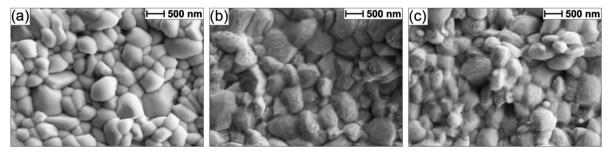
Fig. 2 SEM images for an FTO/Ti/Au/Sb<sub>2</sub>Se<sub>3</sub> sample (a) untreated, (b) etched via (NH<sub>4</sub>)<sub>2</sub>S, and (c) etched via (NH<sub>4</sub>)<sub>2</sub>S + CuCl<sub>2</sub> treatment.
