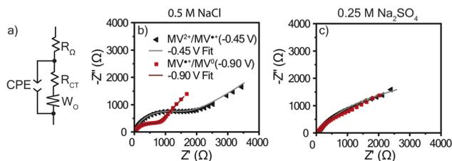
**Fig. 6** (a) The equivalent circuit used to model the EIS data. Nyquist plots for PTPM in (b) 0.5 M NaCl and (c) 0.25 M  $\text{Na}_2\text{SO}_4$  with their curve fits. EIS was conducted at  $-0.45$  V and  $-0.90$  V vs. Ag/AgCl (sat.) with an amplitude of 10 mV in a frequency range of  $5 \times 10^6$  Hz to 0.1 Hz (10 steps per decade). Bode plots are found in Fig. S5 and S6.†
