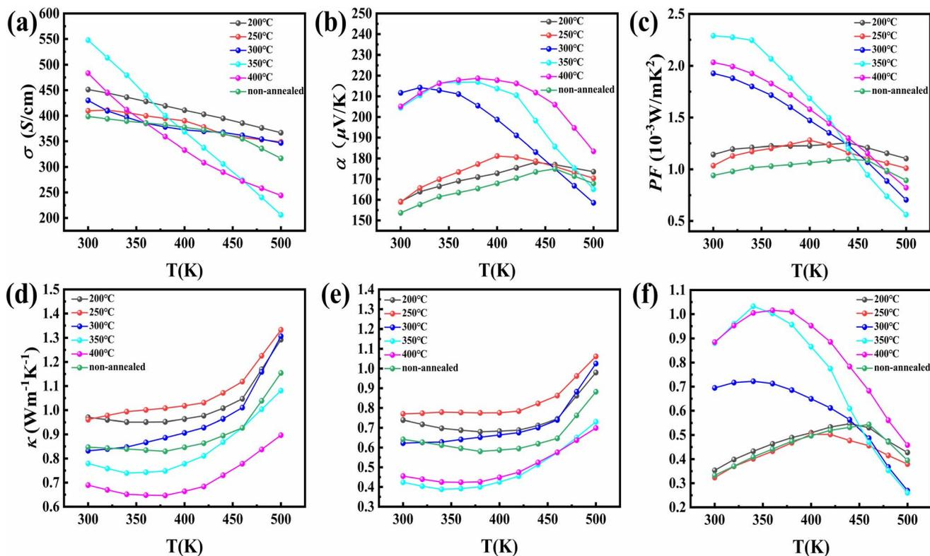
**Fig. 1** Temperature-dependent thermoelectric properties of  $\text{Bi}_{0.5}\text{Sb}_{1.5}\text{Te}_3$  materials under different heat treatment conditions: (a) electrical conductivity, (b) Seebeck coefficient, (c) power factor, (d) thermal conductivity, (e) the combined lattice and bipolar thermal conductivity, and (f)  $ZT$  values.
