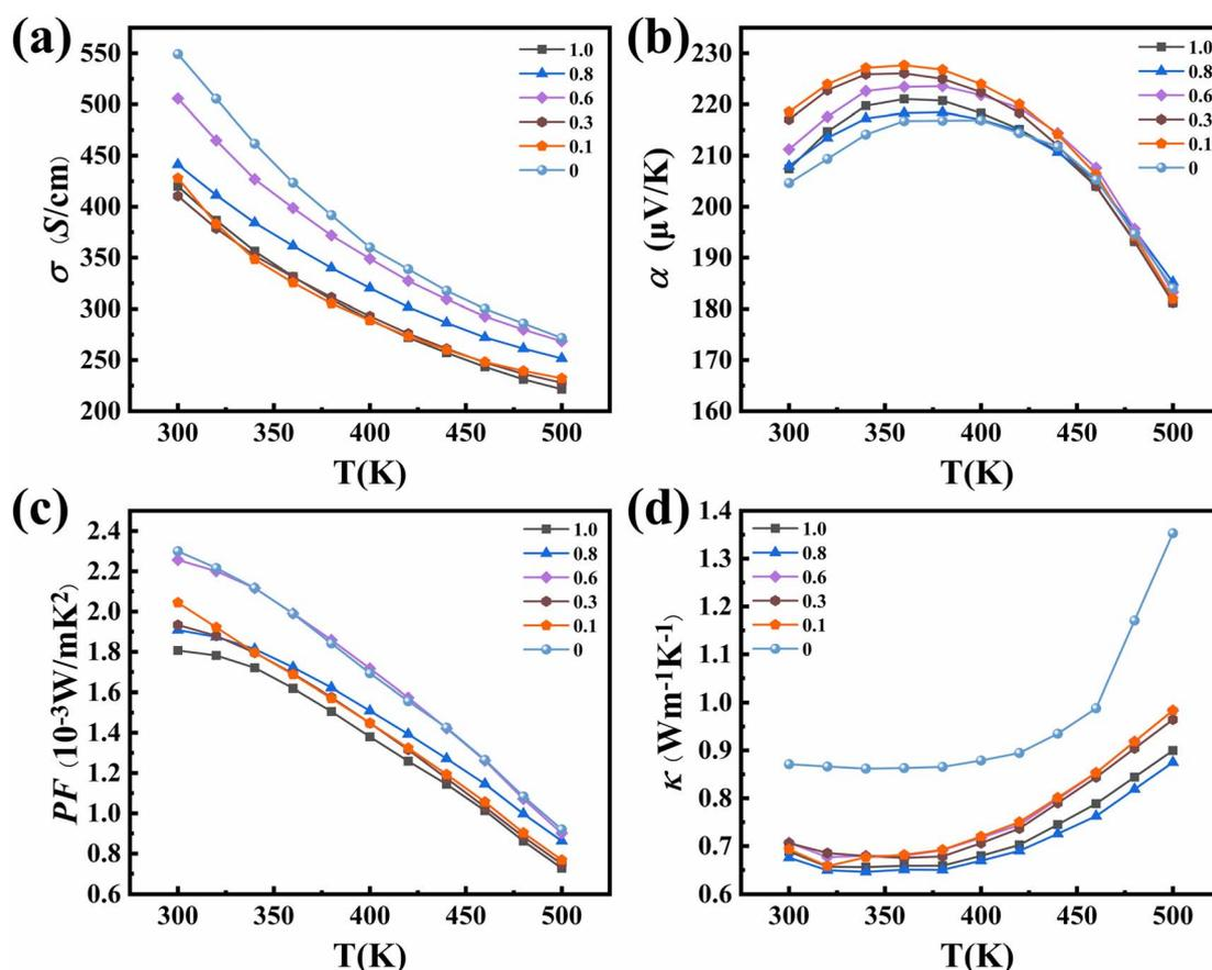
Fig. 5 (a) Electrical conductivity, (b) Seebeck coefficient, (c) power factor, and (d) thermal conductivity of  $\text{Bi}_{0.5}\text{Sb}_{1.5}\text{Te}_3/x\text{vol}\%$  SiC ( $x = 0, 0.1, 0.3, 0.6, 0.8, 1.0$ ) as a function of temperature.
