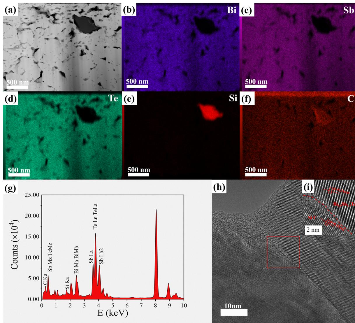
Fig. 4 (a) The microstructure of  $\text{Bi}_{0.5}\text{Sb}_{1.5}\text{Te}_3/x\text{vol}\% \text{SiC}$  ( $x = 0.6$ ), (b–f) the distribution of Si, Bi, Sb and Te elements, (g) EDS composition of  $\text{Bi}_{0.5}\text{Sb}_{1.5}\text{Te}_3/x\text{vol}\% \text{SiC}$  ( $x = 0.6$ ), (h) high-resolution TEM images of  $x = 0.6$  samples, and (i) high-resolution TEM images of  $x = 0.6$  sample interfaces ((i) is the image of the red rectangular area in (h)).
