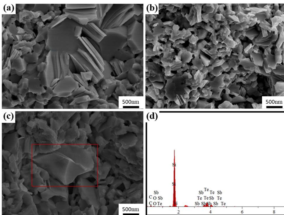
Fig. 3 Fracture morphologies and EDS compositions of  $\text{Bi}_{0.5}\text{Sb}_{1.5}\text{Te}_3/x$  vol% SiC ( $x = 0, 0.6$ ) bulk samples. Fracture morphologies of (a)  $x = 0$  and (b) and (c)  $x = 0.6$  samples; (d) EDS composition of the rectangular area in (c).
