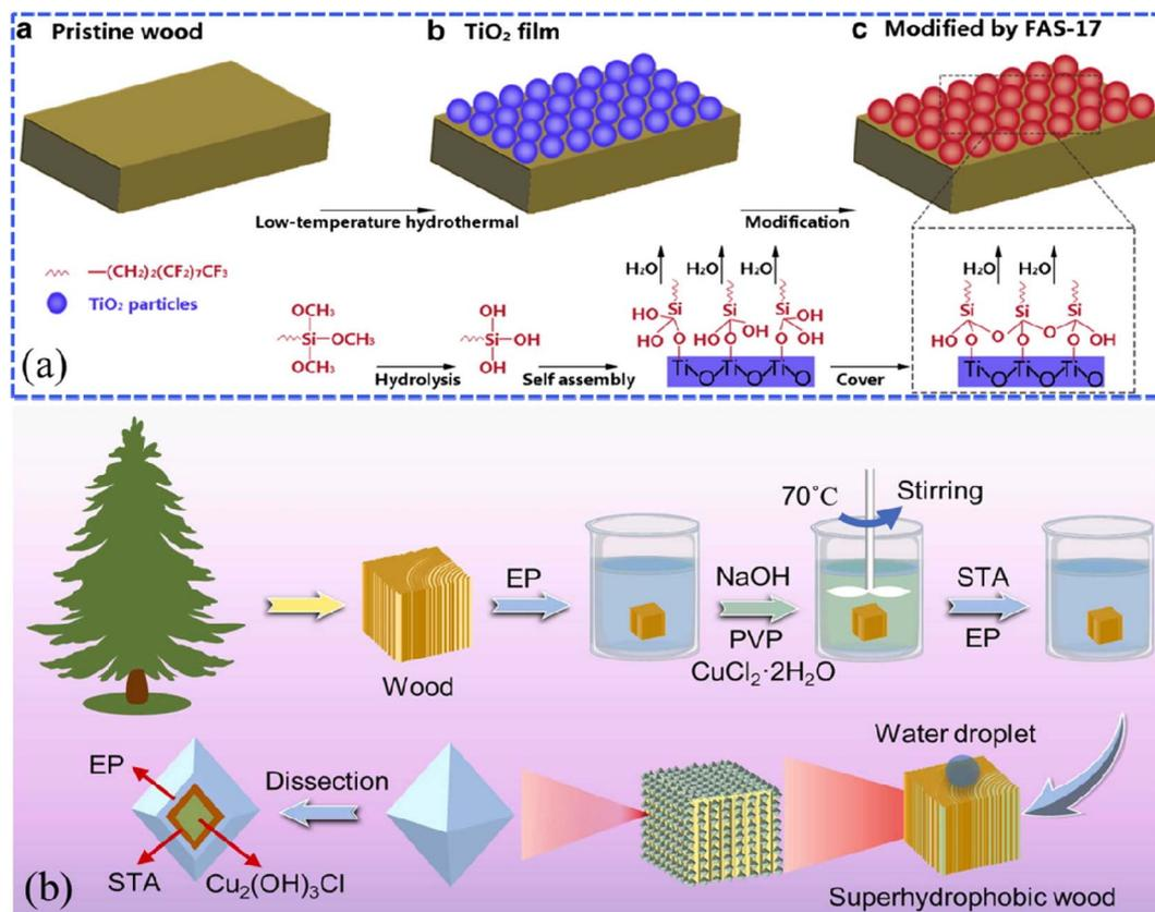
Fig. 4 (a) Schematic illustration of the fabrication of superhydrophobic wood using TiO<sub>2</sub> and (heptadecafluoro-1,1,2,2-tetradecyl)trimethoxysilane (FAS-17). Reproduced with permission from ref. 53. Copyright 2014, Elsevier. (b) A schematic diagram of the *in situ* hydrothermal synthesis of Cu<sub>2</sub>(OH)<sub>3</sub>Cl nanoparticles onto a pine wood surface. Reproduced with permission from ref. 56. Copyright 2022, Elsevier.
