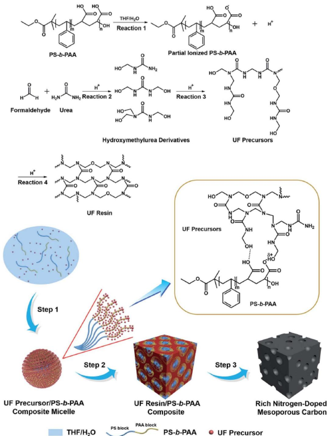
Fig. 4 The formation of rich N-doped mesoporous carbon through a template-catalyzed *in situ* polymerization and co-assembly process.<sup>29</sup> Copyright 2018, Royal Society of Chemistry.
