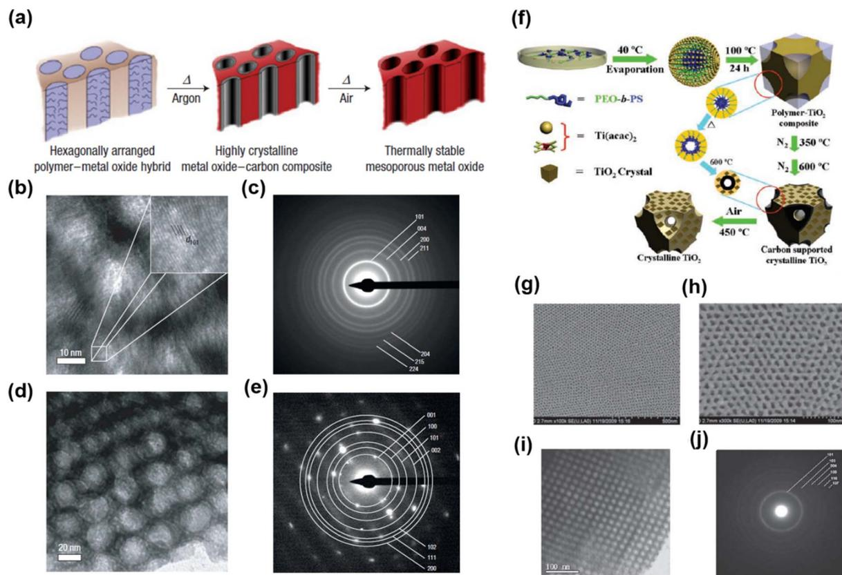
Fig. 5 (a) Schematic of the CASH method. HR-TEM images and SAED patterns of mesoporous  $\text{TiO}_2$  (b, c) and  $\text{Nb}_2\text{O}_5$  (d and e).<sup>137</sup> Copyright 2008, Springer Nature. (f) Process of forming ordered and highly crystallized large-pore mesoporous  $\text{TiO}_2$  from the ligand-assisted assembly method. FESEM (g, h) and TEM (i) images of mesoporous  $\text{TiO}_2$  and its corresponding SAED pattern (j).<sup>68</sup> Copyright 2011, Wiley-VCH.
