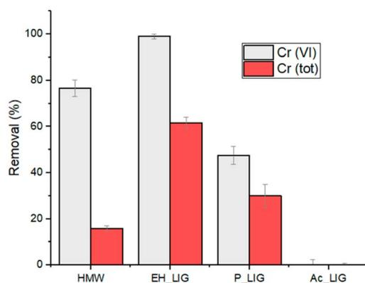
Fig. 8 Cr(tot) removal and Cr(vi) reduction by using different types of lignin at pH 2 ( $2 \text{ M HNO}_3$ ).  $1 \text{ g L}^{-1}$  of lignin; initial Cr(vi) concentration:  $5 \text{ mg L}^{-1}$ ; contact time: 2 h.
