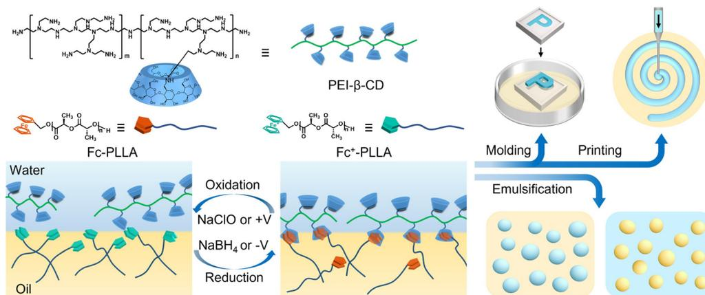
**Fig. 1** Schematic representation of the assembly/disassembly of PEIS at the oil–water interface in a redox process, and the preparation of liquid letter, liquid spiral and different types of emulsions.
