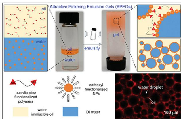
Fig. 4 The formation mechanism and fluorescence confocal microscope image of APEGs.<sup>4</sup> Copyright 2021 Wiley.
