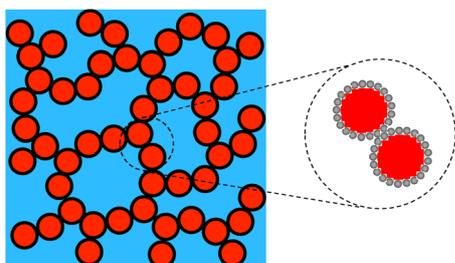
Fig. 2 Schematic representation of emulsion particulate gels.
