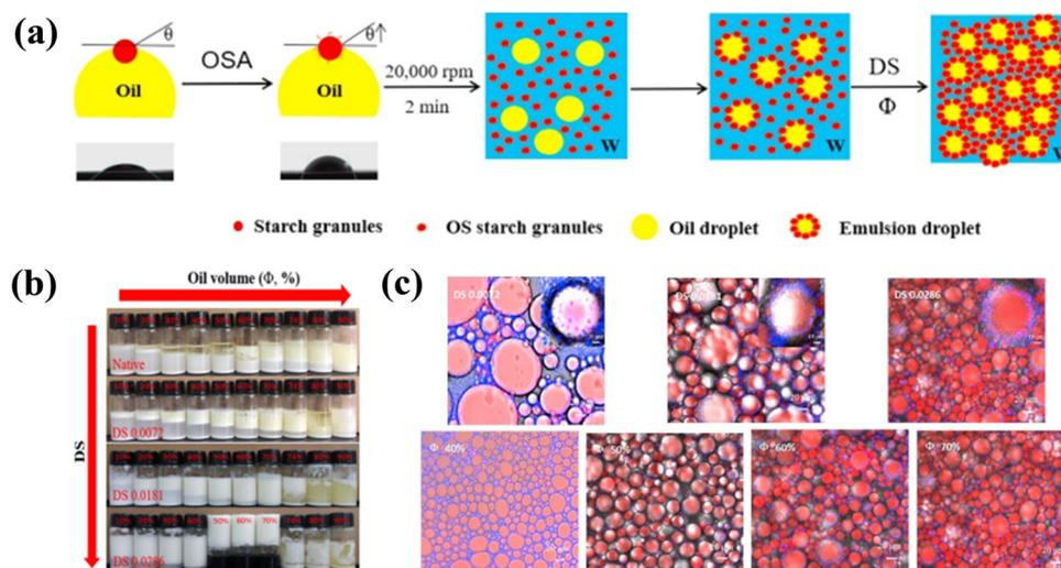
**Fig. 6** (a) Mechanism of formation of OS quinoa starch-based Pickering emulsion gels as a function of the degree of substitution (DS) and oil volume fraction ( $\phi$ ). (b) The visual appearance of Pickering emulsions stabilized by native and OS quinoa starches as a function of DS and  $\phi$ . (c) Confocal microscopy images of Pickering emulsions and emulsion gels stabilized by OS quinoa starches as a function of DS and  $\phi$ .<sup>22</sup> Copyright 2019 Elsevier.
