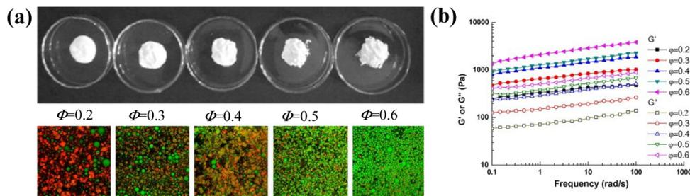
Fig. 3 (a) Visual images of heat-treated WPC emulsions at various oil fractions ( $\Phi = 0.2$ – $0.6$ ) after 1 day storage at room temperature. The bottom row shows the confocal laser scanning microscopy images of the emulsions. The dimension for the images is  $7.5 \times 7.5 \mu\text{m}$ . (b) Variations of  $G'$  and  $G''$  with frequency at  $25^\circ\text{C}$  for the heat-treated WPC emulsions at various oil fractions ( $\Phi = 0.2$ – $0.6$ ).<sup>17</sup> Copyright 2011 Elsevier.
