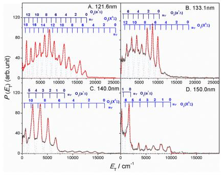
Fig. 2 The product total kinetic energy ( $P(E_T)$ ) spectra for  $S(^1D) + O_2$  products following photolysis at  $\lambda = (A)$  121.6 nm, (B) 133.1 nm, (C) 140.0 nm and (D) 150.0 nm, derived from the images shown in Fig. 1, in red, along with the best-fit simulation of the spectra, in cyan dashed lines and orange dotted lines. The superposed combs indicate the  $E_T$  values associated with the formation of the various vibrational levels of  $O_2(X^3\Sigma_q^{-})$  $a^1\Delta_g$ , v).
