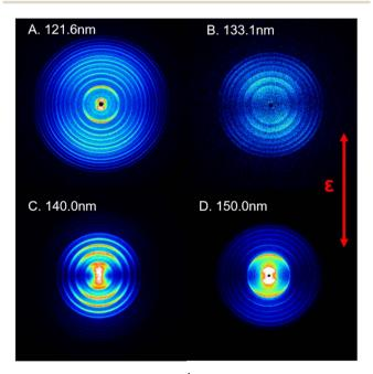
Fig. 1 Time-sliced images of the S( $^1$ D) products from SO $_2$  photodissociation. The images were recorded at photolysis wavelengths  $\lambda=$  (A) 121.6 nm, (B) 133.1 nm, (C) 140.0 nm and (D) 150.0 nm. The double headed red arrow indicates the polarization direction of the photodissociation laser,  $\varepsilon$ . The concentric ring features reflect the population of different vibrational levels of the coincident  $O_2(X^3\Sigma_{\alpha}^{-}/a^1\Delta_{\alpha}, \nu)$  products.
