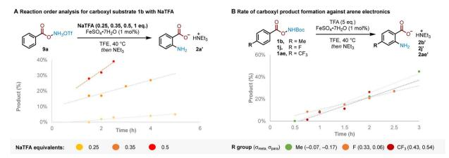
Fig. 2 (A) Reaction order analysis in NaTFA for triflate salt 9a. (B) Rate-determining step (RDS) inference from rate of product formation with varying arene electronics. Yields determined by  $^1H$  NMR using 1,2-DME as an internal standard after quenching with  $Et_3N$  and filtering through silica.
