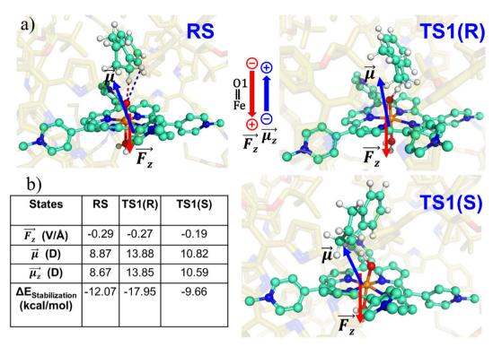
Fig. 8 (a) RS, TS1-R and TS1-S states showing the direction of local electric field (LEF) and dipole moment. (b) Calculated LEF<sub>z</sub>, dipole moments, and stabilization energies. Note that we have a GAUSSIAN convention to define the direction of electric fields and dipole moments. Dipole moments have been calculated for H<sub>2</sub>O-Fe=O, porphyrin and TLN.
