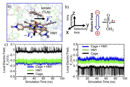
Fig. 4 (a) A representative MD snapshot highlighting the reactive complex inside the cage. (b) Reaction axis & electric field direction, GAUSSIAN convention is used. (c) The local electric field (LEF) along y- and z-axis with evolution of time.
