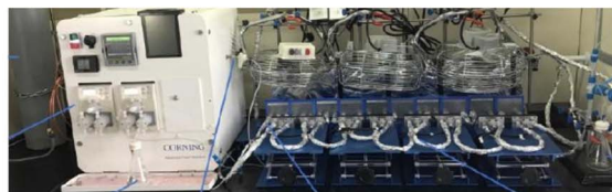
A: Cerium photocatalysis enabled alkane amination in continuous flow
