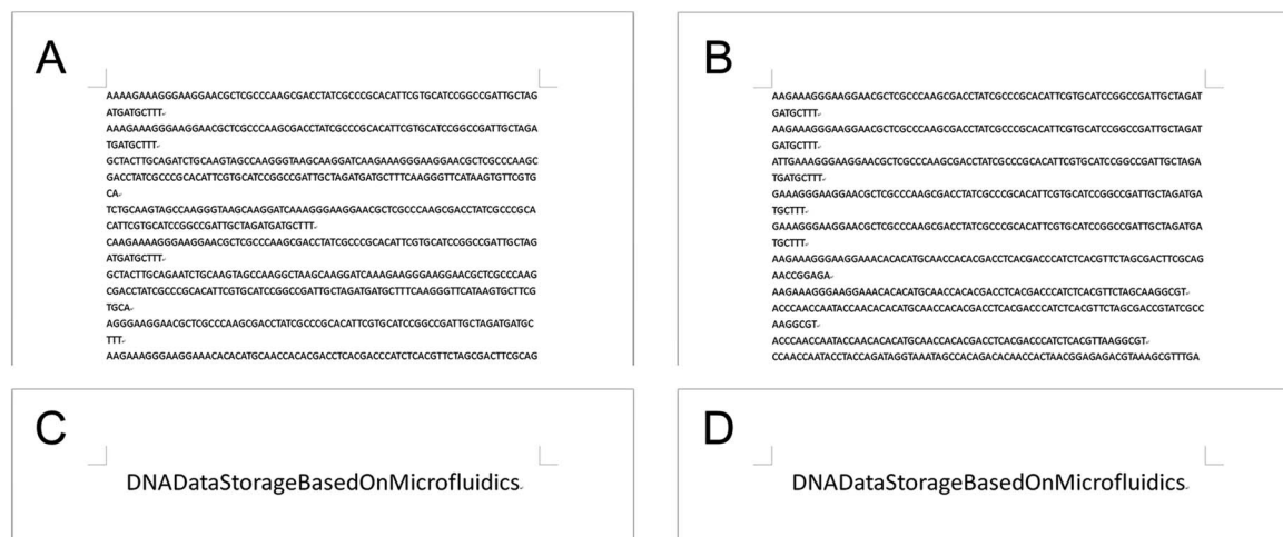
Fig. 5 Text information extraction from mineralized DNA data off-chip and on-chip. (A) The partial results of high-throughput sequencing (off-chip). (B) The partial results of high-throughput sequencing (on-chip). (C) The decoding text information from the results of high-throughput sequencing (off-chip). (D) The decoding text information from the results of high-throughput sequencing (on-chip).
