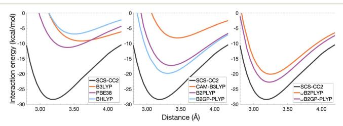
Fig. 8 Dissociation energy curves of the lowest-lying singlet excited state of the fully-stacked anthracene dimer.
