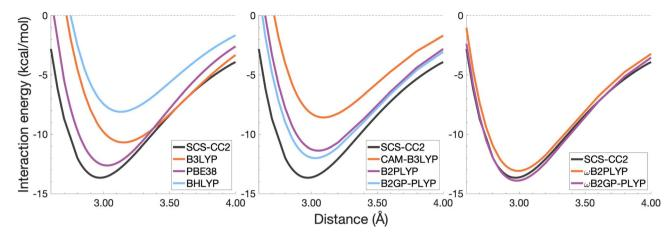
Fig. 6 Dissociation energy curves of the lowest-lying singlet excited state of the fully-stacked benzene dimer.
