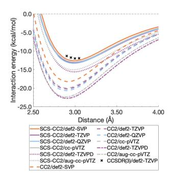
**Fig. 3** Benzene excimer dissociation curves for various CC2 and SCS-CC2 based levels of theory compared to select CCSDR(3)/def2-TZVP points.
