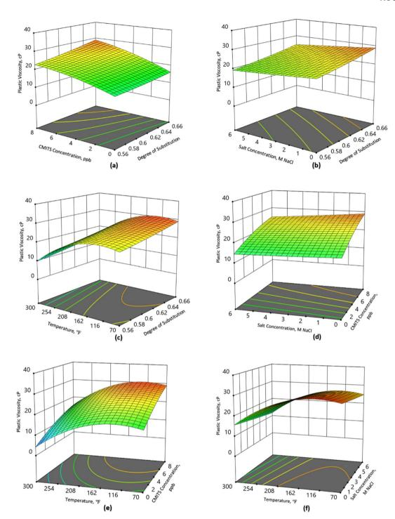
Fig. 2 Influence of (a) DS and CMITS dosage, (b) DS and salt dosage, (c) DS and temperature, (d) CMITS and salt dosage, (e) CMITS dosage and temperature, and (f) salt dosage and temperature on the plastic viscosity.
