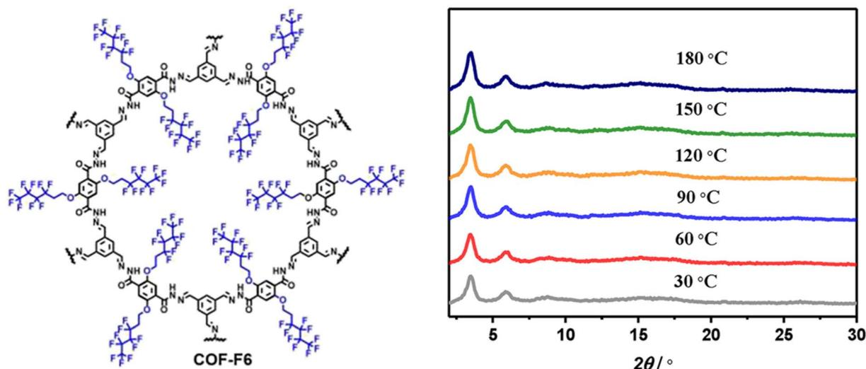
Fig. 4 Structure of COF-F6 and the corresponding PXRD pattern at various temperature. Reprinted with permission,<sup>52</sup> Copyright (2020) from American Chemical Society.
