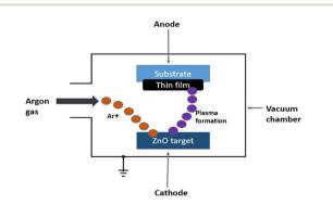
Fig. 16 A schematic of the ZnO RF magnetron sputtering system.
