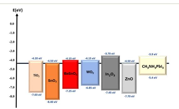
Fig. 7 A summary of the energy levels of metal oxide materials as ETL and perovskite.
