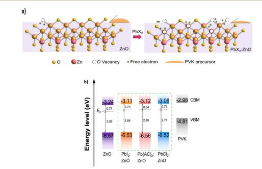
Fig. 22 (a) Energy level alignment of ETLs and the perovskite layer. (b) Visualization of the impact of the enhanced oxygen vacancy in PbX<sub>2</sub>:ZnO. This figure has been reproduced from ref. 136 with permission from Wiley, copyright 2022.
