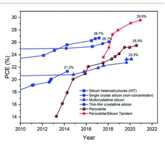
**Fig. 2** The evolution of silicon, perovskite, and perovskite–silicon tandem device efficiency over the past decade, as derived from the efficiency table published by the National Renewable Energy Laboratory. This figure has been reproduced from ref. 2 with permission from the Royal Society of Chemistry, copyright 2021.
