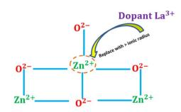
Fig. 18 A schematic image of the  $ZnO^{2+}$  cation substitution or passivation in the doping engineering process with lanthanum as an addictive dopant.
