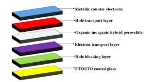
Fig. 5 A generic structure of PSC for achieving the optimal efficiency based on the energy levels of materials from each layer.
