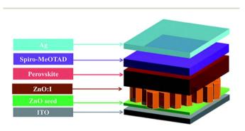
**Fig. 21** A schematic illustration of the PSC configuration, in which a dense and homogeneous perovskite cap layer completely covers the ZnO:I nanopillars. Reproduced with permission from ref. 125. Copyright 2017 Royal Society of Chemistry.
