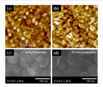
Fig. 9 Material images of (a) AFM for bare  $SnO_2$ , (b) AFM for Ni-doped  $SnO_2$ , (c) SEM for bare  $SnO_2$ , and (d) SEM for Ni-doped  $SnO_2$ . Reproduced with permission from ref. 57. Copyright 2022 American Chemical Society.
