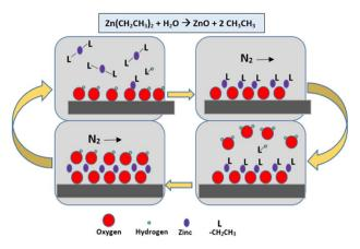
Fig. 17 A schematic illustration of ZnO atomic layer deposition synthesis.
