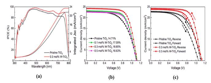
Fig. 11 (a) IPCE curves of pristine TiO<sub>2</sub> and 0.3% mol W-doped TiO<sub>2</sub>. (b) IV curve of PSC with different W concentrations. (c) Reverse and forward direction of the IV curve. Reproduced with permission from ref. 78. Copyright 2021 Elsevier.
