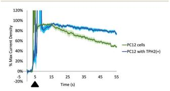
Fig. 7 Normalized current density (to the maximum current in each curve, excluding those signals called by mechanical noise from the injection itself) for exogenously applied 10  $\,\mu L$  of 5  $\,\mu M$  Trp (black triangle) to cultured PC-12 cells (green, n=5 measurements) and PC-12 cells with overexpressed tryptophan hydroxylase 2 (TPH2(+), n=6 measurements). Pale blue and pale green error bars indicate SEM. \*\*\*\*p<0.0001. Time resolution was 100 ms.
