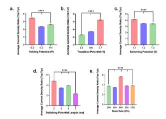
Fig. 3 Plot of ratios of current densities of Trp to Tyr as an indicator of selectivity for the different optimized parameters: (a) holding potential, (b) transition potential, (c) switching potential, (d) duration of switching potential, and (e) scan rate. Error bars are  $\pm$ SEM. \*\*\*\*p < 0.0001.
