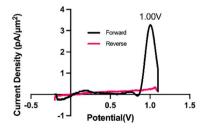
Fig. 1 Representative cyclic voltammogram for Trp oxidation on carbon fiber microelectrode using the multi-scan rate waveform. Black trace indicates the forward scan while the red trace indicates the reverse scan. The primary oxidation peak occurs at 1.00 V.
