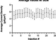
Fig. 6 Average current density over 25 consecutive injections (error bars = SEM).
