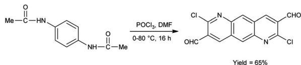
Scheme 49 Synthesis of 2,7-dichloropyrido[2,3-g]quinoline-3,8-dicarbaldehyde.
