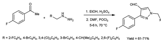
Scheme 8 Synthesis of 1-substitutedbenzyl-3-(4-fluorophenyl)-1H-pyrazole-4-carbaldehydes.
