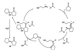
Fig. 26 Self-aldol condensation of cyclopentanone
