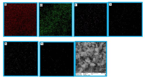
Fig. 4 Elemental mapping images of the KIT-6@SMTU@Ni catalyst.
