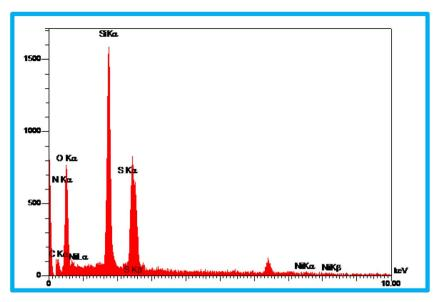
Fig. 3 The EDS spectrum of the KIT-6@SMTU@Ni catalyst.
