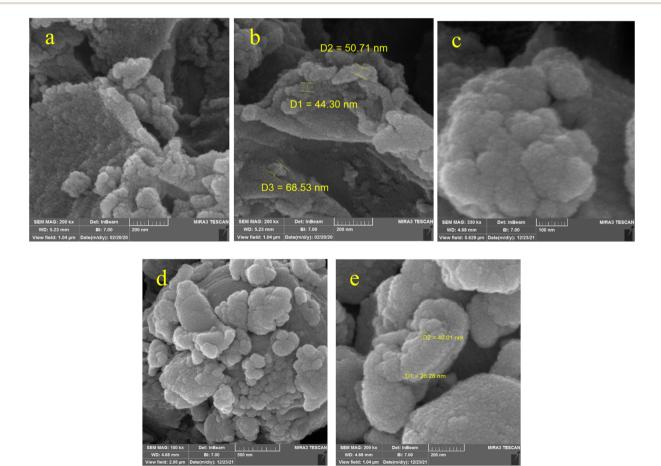
Fig. 2 SEM images of (a and b) KIT-6 and (c-e) the KIT-6@SMTU@Ni catalyst.
