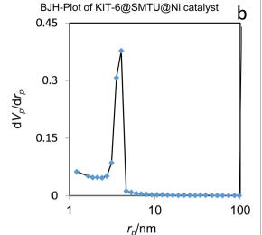
Fig. 8 BJH diagrams of KIT-6 (a) and the KIT-6@SMTU@Ni catalyst (b).
