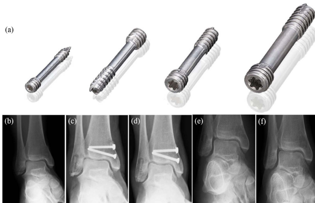
Fig. 5 (a) MAGNEZIX® compression screws: from left to right: MAGNEZIX® CS 2.0, MAGNEZIX® CS 2.7, MAGNEZIX® CS 3.2, MAGNEZIX® CS 4.8. (b–f) X-ray of ankle fracture: (b) ankle fracture type AO–ASIF 44–A2.3; before surgery (c) six weeks after surgery; (d) 3 months after surgery; (e) 8 months after surgery, metal removal; (f) 17 months after surgery. 81
