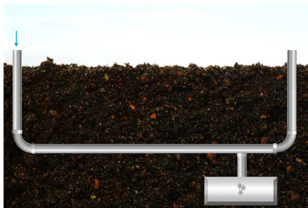
Fig. 13 Schematic of condensation drinking water production method.
