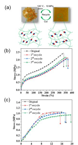
Fig. 4 Schematic representation of reprocessing of vitrimer (a); tensile test of FDV-1071 (b) and SCV-1071 (c).
