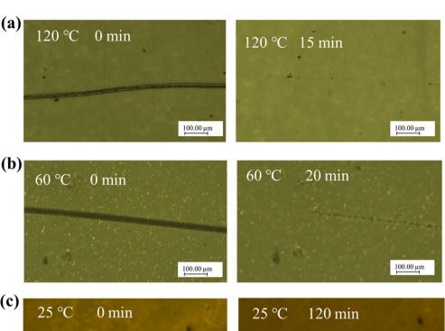
Fig. 7 Optical microscopy images of scratched FDV-1071 (a) at 120 °C, (b) at 60 °C, and (c) at 25 °C.
