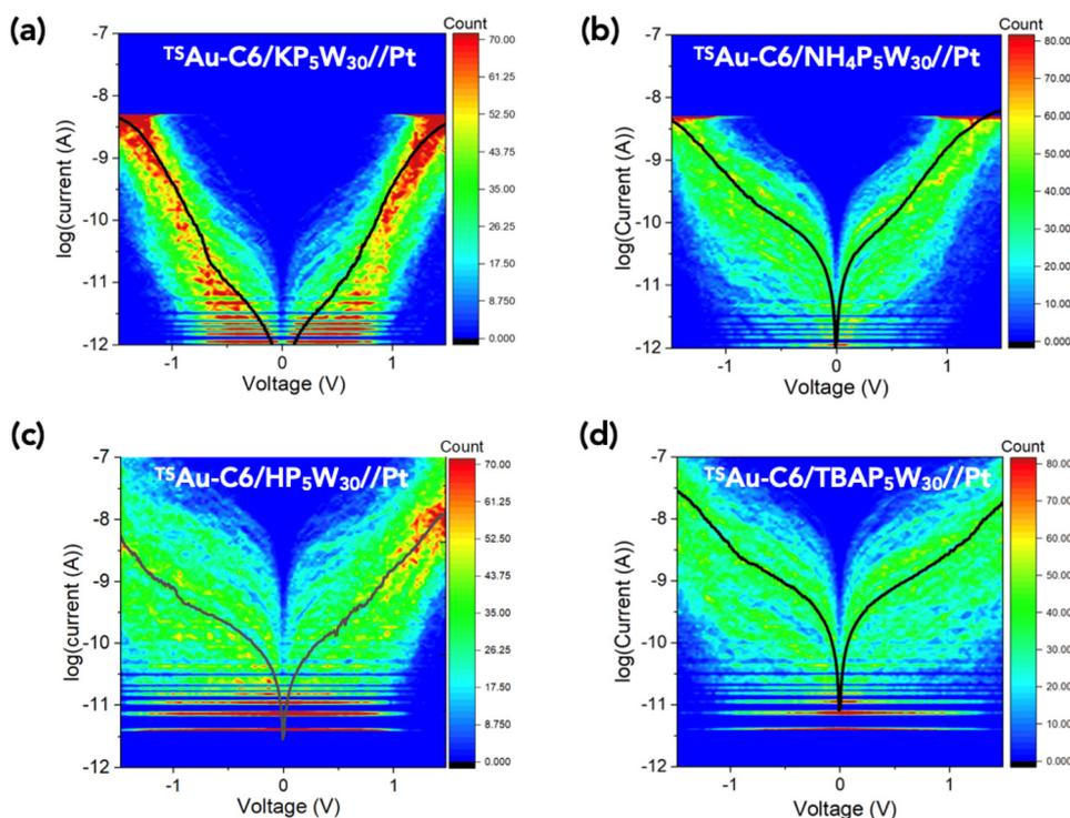
**Fig. 2** 2D histograms (400–500  $I$ - $V$  traces) of the four samples in a semi- $\log|I|$ - $V$  plot. The solid black lines are the calculated mean  $\bar{I}$ - $V$  curves. (a)  $KP_5W_{30}$  MJs, (b)  $NH_4P_5W_{30}$  MJs, (c)  $HP_5W_{30}$  MJs and (d)  $TBAP_5W_{30}$  MJs.
