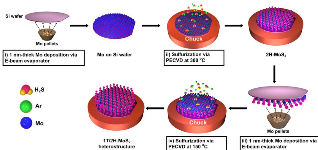
**Scheme 1** Synthesis steps of the vertical stacking of 1T- and 2H-MoS<sub>2</sub> on Si substrates using a 13.56 MHz ICP plasma process.
