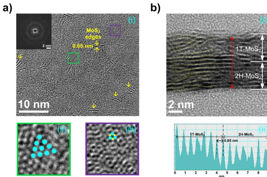
Fig. 2 (a) HRTEM top view and (b) HRTEM cross-sectional image of the 1T/2H-MoS<sub>2</sub> vertical heterostructure.
