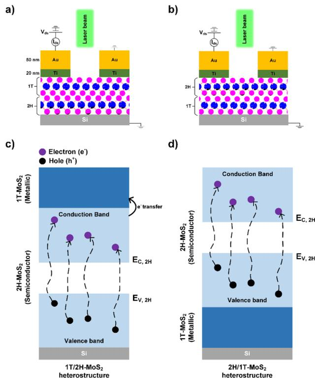
**Scheme 2** Cross-sectional view of (a) 1T/2H-MoS<sub>2</sub> and (b) 2H/1T-MoS<sub>2</sub> photodetector structures. The corresponding electron–hole pair generation mechanism for (c) 1T/2H-MoS<sub>2</sub> and (d) 2H/1T-MoS<sub>2</sub>.
