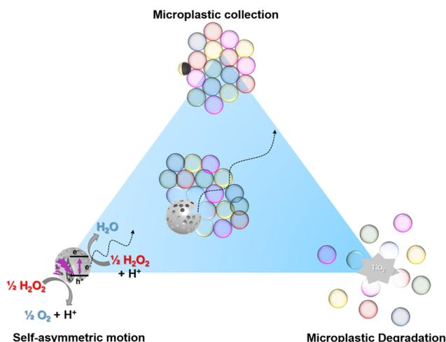
**Fig. 1** Schematic illustration of our current photocatalytic micromotor-based system (at center) combining the principles of inherently self-asymmetric motion (bottom left), micromotor-based collection of microplastic (top), and photocatalytic degradation of microplastics (bottom right). The colorful translucent spheres represent polystyrene microparticles, and the transparent ones close to the photocatalyst (right and center) are degraded due to the photocatalytic action.
