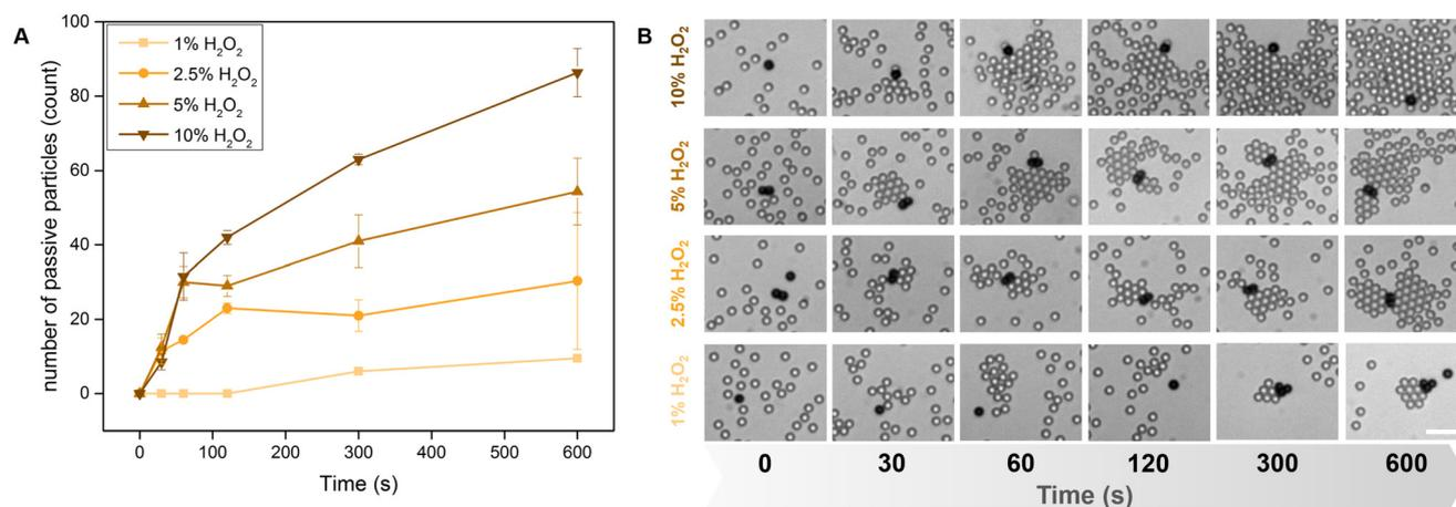
**Fig. 3** (A) Quantification of rafting behavior with SiO<sub>2</sub> colloids and (B) optical microscopy snapshots after different time intervals at different H<sub>2</sub>O<sub>2</sub> concentrations. A UV light of intensity 19.08 W cm<sup>-2</sup> and wavelength 385 nm is used.
