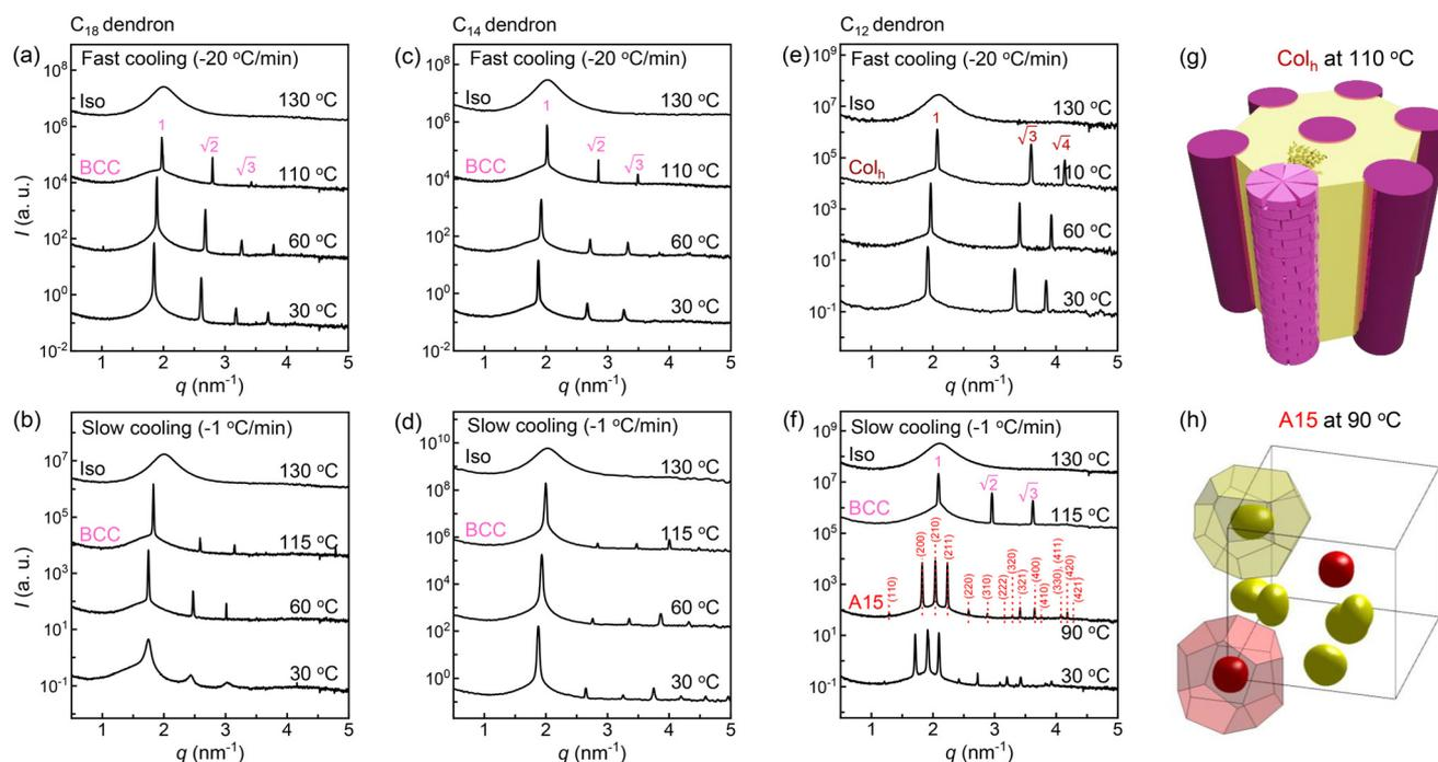
**Fig. 2** SAXS intensity profiles of (a and b)  $C_{18}$ , (c and d)  $C_{14}$ , and (e and f)  $C_{12}$  dendrons with two different cooling rates of  $-20$  and  $-1$  °C min<sup>-1</sup> from 130 to 30 °C. 3D morphologies reproduced from the ED maps of (g) the stacked Col<sub>h</sub> and (h) A15 phases, which are obtained from the fast and slow cooling of the  $C_{12}$  dendrons, respectively.
