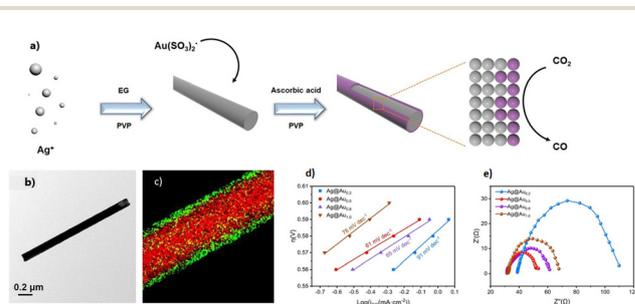
**Fig. 4** (a) Schematic preparation process of Ag@Au core-shell nanowires. (b) Representative TEM image. (c) HAADF-STEM elemental mapping. (d) Tafel slope of Ag@Au<sub>0.2</sub>, Ag@Au<sub>0.5</sub>, Ag@Au<sub>0.8</sub> and Ag@Au<sub>1</sub> electrocatalysts. (e) EIS characterization of Ag@Au<sub>0.2</sub>, Ag@Au<sub>0.5</sub>, Ag@Au<sub>0.8</sub> and Ag@Au<sub>1</sub> electrocatalysts.
