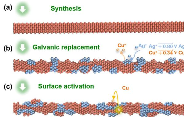
Fig. 3 (a) Starting CuNWs. (b) Galvanic replacement on the surface. (c) Surface activation through *in situ* formation of CuAg assemblies during the electrochemical CO<sub>2</sub>RR. Reproduced with permission from ref. 57. Copyright 2021, Springer.
