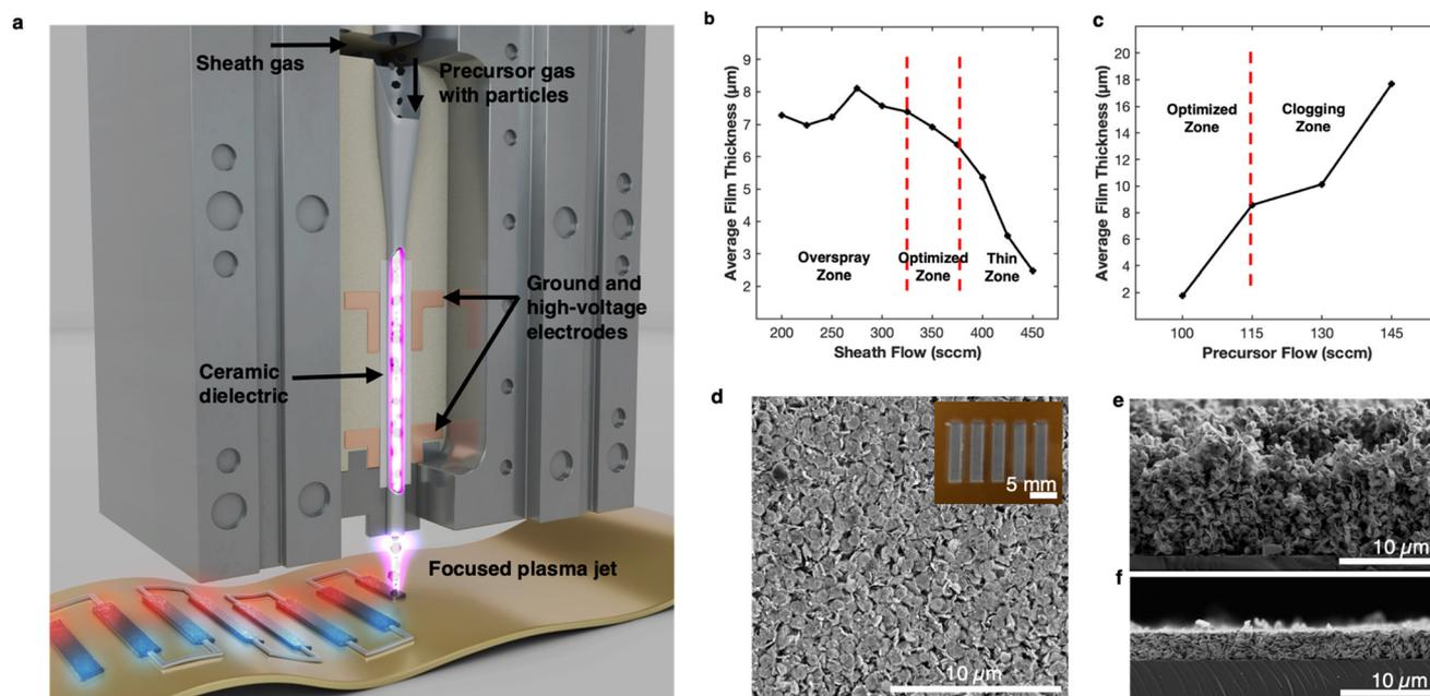
**Fig. 2** Print and film optimization. (a) Schematic diagram of the PJP printhead. Average thickness by (b) sheath flow and (c) precursor flow showing optimized conditions. (d) Top-down scanning electron microscopy image of the printed film (inset) after mechanical pressing. Cross sectional SEM of the printed film (e) as printed and (f) after pressing and sintering.
