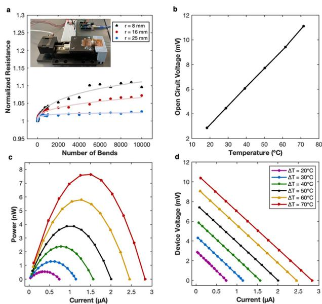
**Fig. 5** Electrical characterization of single leg TE film sintered at 425 °C. (a) Resistance as a function of bending cycles for various radii of curvature. Inset shows bending test apparatus. (b) Open circuit voltage as a function of temperature difference, (c) device voltage as a function of current and (d) power curves for several temperature differentials.
