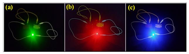
Fig. 6 (a) Photograph of the green LED with two NH-CNPS-rGO-2||AC devices connected in series. (b) Photograph of the red LED with two NH-CNPS-rGO-2||AC devices connected in series. (c) Photograph of the blue LED with two NH-CNPS-rGO-2||AC devices connected in series.
