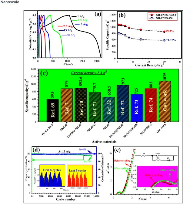
Fig. 4 (a) GCD plots of the NH-CNPS-rGO-2 electrode from 1 to 30 A  $g^{-1}$ . (b) Specific capacities vs. current densities of the NH-CNPS-rGO-2 and NH-CNPS-350 electrodes. (c) Comparison of capacity values of NH-CNPS-rGO-2 with the results previously reported in the literature. (d) Longevity and coulombic efficiency of NH-CNPS-rGO-2 at 15 A  $g^{-1}$  (the inset illustrates the first and last 5 GCD cycles). (e) Nyquist curves of NH-CNPS-rGO-2 before and after 13 000 GCD cycles.
