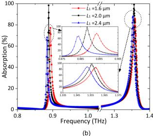
Fig. 5 Absorption spectra of the metamaterial absorber under normal TE polarization with (a) parameter a ranging from 20.2 to 21.8  $\mu$ m, (b) parameter  $L_1$  changing from 1.6 to 2.4  $\mu$ m, (c) parameter  $L_2$  shifting from 23.3 to 24.9  $\mu$ m, (d) parameter  $W_1$  increasing from 0.2 to 1.8  $\mu$ m and (e) parameter  $W_2$  growing from 1.5 to 2.5  $\mu$ m.
