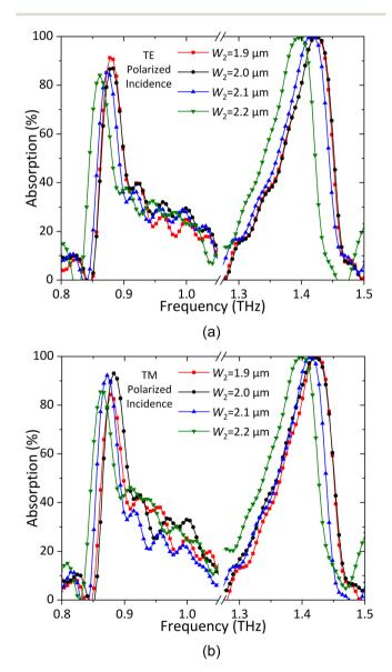
Fig. 8 Measurement results of the fabricated dual-band metamaterial absorbers with different values of  $W_2$  under (a) normal TE polarized incidence and (b) normal TM polarized incidence.
