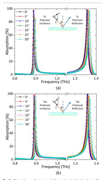
Fig. 6 Absorption performance of the metamaterial absorber with a change in the incident angle from 0° to 30° of the (a) absorption spectra under TE polarized incidence, (b) absorption spectra under TM polarized incidence, (c) Q-factors under TE polarized incidence, and (d) Q-factors under TM polarized incidence. (e) Absorption spectra with a shifting polarization angle from 0° to 90°.
