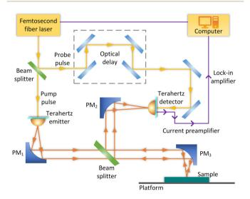
Fig. 7 Schematic diagram of the terahertz TDS measurement system.
