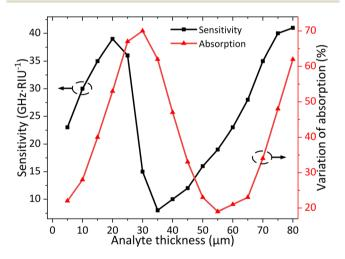
Fig. 10 Sensitivity and variation of absorption with the analyte thickness ranging from 5 to 80  $\mu m. \,$
