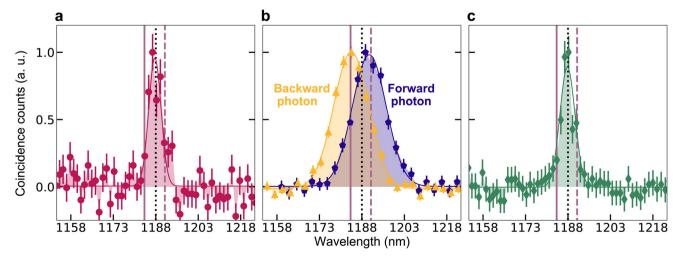
Fig. 3 The SPDC spectra for (a) forward-forward, (b) forward-backward, and (c) backward-backward measurement. Solid lines are Gaussian fits. Vertical solid and dashed lines in the graphs indicate the resonance wavelength and the wavelength related to it through the energy conservation condition. Vertical dotted lines show the degenerate wavelength.
