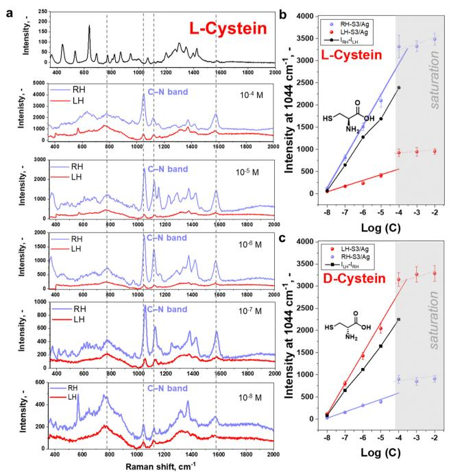
Fig. 2 (a) Stacked SERS spectra of L-cysteine enantiomer deposited on LH- or RH-S3/Ag substrates from methanol solutions with various initial concentrations ( $10^{-4}-10^{-8}$  M range) measured at 785 nm; (b) and (c) the characteristic L-cysteine and D-cysteine SERS band ( $1044 \text{ cm}^{-1}$ ) intensity as a function of the initial enantiomers concentrations and plasmonic substrate LH- or RH-kind.
