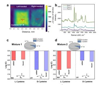
Fig. 3 (a) SERS mapping of D-cysteine ( $10^{-5}$  M) on RH- and LH-S3/Aq structures measured at 785 nm; (b) stacked SERS spectra from local points, designated on (a); (c) measured at 785 nm, (d) example of enantiomers content determination in L/D-cysteine mixtures using measurements on LH- and RH-S3/Ag SERS substrates.
