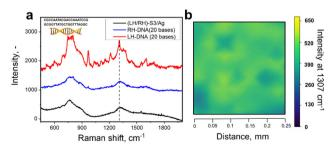
Fig. 5 (a) Stacked SERS spectra of double-stranded DNA measured on LH- and RH-S3/Ag substrates measured at 785 nm, bottom spectrum (black) shows the "background" signal from pristine LH-S3/Ag substrate; (b) SERS mapping of double-stranded DNA obtained across the LH-S3/Ag substrate measured at 785 nm
