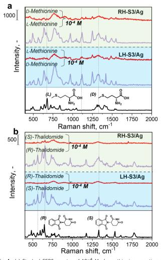
Fig. 4 (a) Stacked SERS spectra of  $10^{-4}$  M L/D-methionine enantiomer deposited on LH- or RH-S3/Ag substrates from methanol solutions measured at 785 nm, (b) SERS spectra of  $10^{-4}$  M (R)/(S)-thalidomide enantiomer deposited on LH- or RH-S3/Ag substrates from methanol solutions measured at 780 nm measured at 785 nm. Bottom spectra (black) show Raman spectra of both compounds
