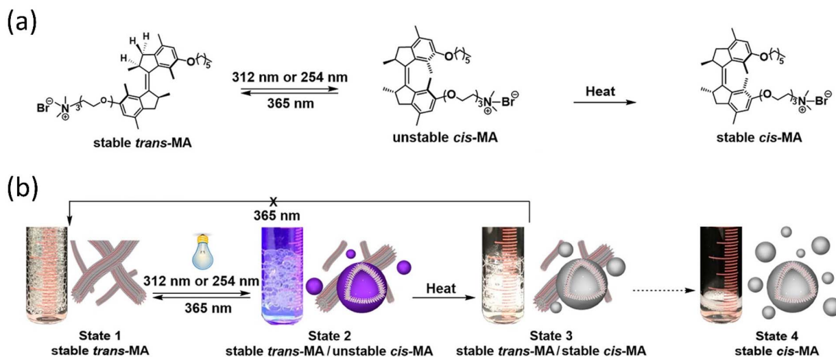
Fig. 9 (a) Light-responsive molecular motor amphiphile (MA) and its reversible photoisomerization process. (b) The alteration in visible macroscopic foaming processes brought structural changes in the supramolecular assembly. Stable synthetically purified cis -MA is used to create state 4. Reproduced with permission. 144 Copyright 2020, American Chemical Society.
